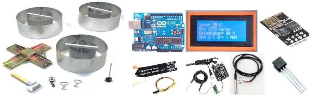
Gambar 1. Double Ring Infiltrometer & Sensors
